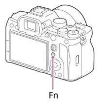
3 Press the top/bottom/left/right side of the control wheel to select a function to set.
